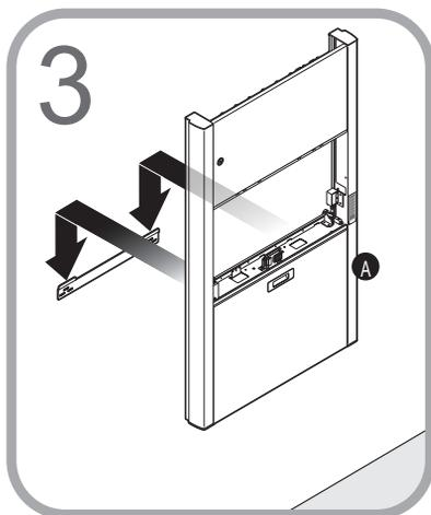
Hang the wall cabinet (A) onto the wall cleat.
