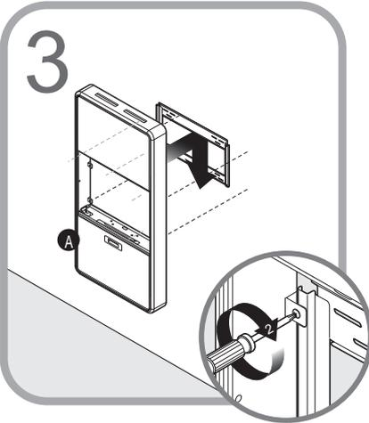
Hang wall cabinet (A) on wall cleat and secure with screws.
