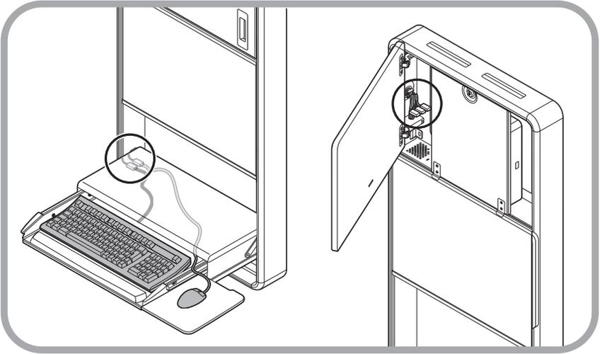
Two USB cables are located in the rear corner of the keyboard tray. These are routed to the technology box area and should be plugged into the CPU.
