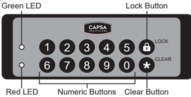
In normal operation the user will enter a 4-digit access code. Once a numeric key is pressed, the green LED will light. The user will then enter the remaining 3-digits of their code. If the access code is accepted, the green LED will blink and the door actuator will be released for the time period specified. If the password is not accepted, the red LED will blink.
