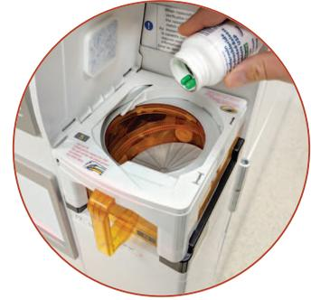
Cassettes can only be opened while docked at the Cassette Station, and by an authorized user. FillSafe system prevents accidental mis-fills and unauthorized access.
