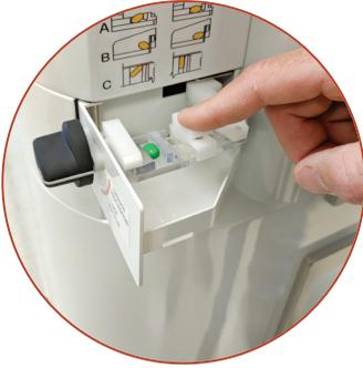
The KL108 Camera Chamber takes precise measurements of each tablet or capsule to auto-calibrate each cassette, eliminating human error.
