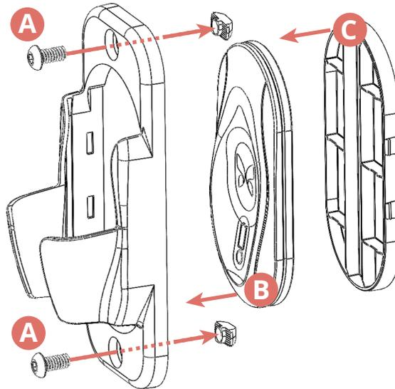
4. Insert the Z-nuts into the channel on the pole.
