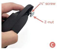
4. Insert the Z-nuts into the channel on the front of the pole.
