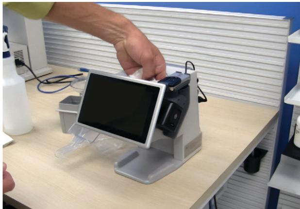
The counting sensors are located behind the four glass windows inside the body of the unit, under the funnel and channel (**C** in Figure 30). Most counting errors are caused by an accumulation of pill dust on the edges and corners of these windows.
